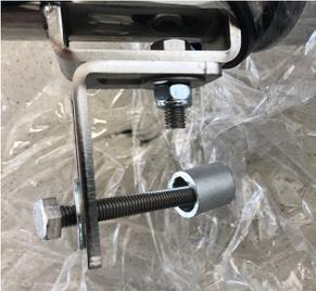
A photograph showing a metal plate being secured to a metal frame. A bolt is being inserted through a hole in the plate and tightened against the frame.                 | Fixations latérales du porte-plaque |
