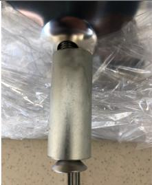
A close-up photograph showing a cylindrical metal component being inserted into a hole in a metal plate. The component has a threaded end and a smooth, tapered section. | Fixation centrale du porte-plaque   |
